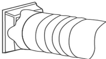
**Step 2:** Connect the windows kit adapter to the other end of the exhaust hose.
