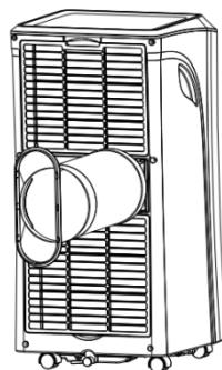
**Step 6:** Adjusting the length of the flexible exhaust hose and avoid bends in the hose. Then place AC near an electrical outlet.
