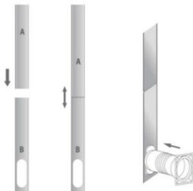
**Step 4:** Close your window to secure the kit in place. It needs to hold the windows kit firmly in place, secure the window kit with duct tape if required. It is recommended that the gap between the adapter and the sides of the window should be sealed off for maximum efficiency.
